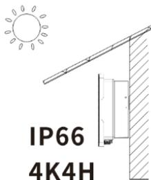
5. The mounting condition must be suitable for the weight and size of the inverter. The inverter is suitable to be mounted on solid wall that is vertical or tilted backwards (Max. 15°). It is not recommended to install the inverter on the wall made of plasterboards or similar materials. The inverter may make noise when working.
