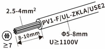
2. Crimp the contacts with the corresponding cables. Crimping tool: H4TC0001, AMPHENOL
