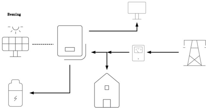
3) When GRID failure and PV energy is insufficient, the battery supplies power to the load.
