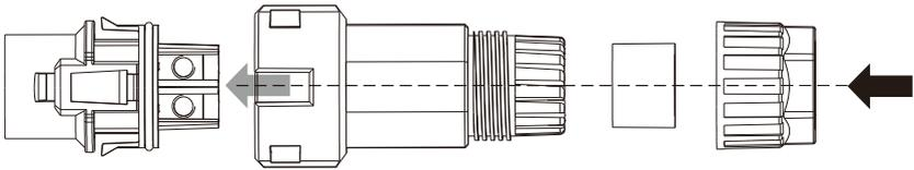
4. Insert the crimped conductors L, N and PE into the corresponding terminals and tighten the screw with a accompanied Torx screwdriver(TX 8, torque: 1.4Nm). Ensure that all conductors are securely in place in the screw terminals on the bush insert. Assemble the locking cap, threaded sleeve and swivel nut together.
