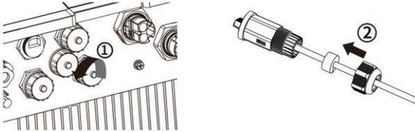
3) Insert the network cable into the corresponding communication terminal of the machine according to the arrow sequence, tighten the thread sleeve, and then tighten the forcing nut at the tail.
